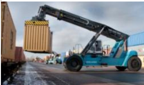
Photograph 1: Reachstacker Lifting an ISO Container
