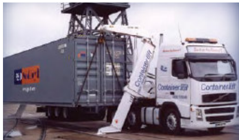
Photograph 1: Reachstacker Lifting an ISO Container
