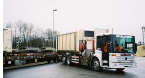
Photograph 3: Side Lift vehicle in operation
